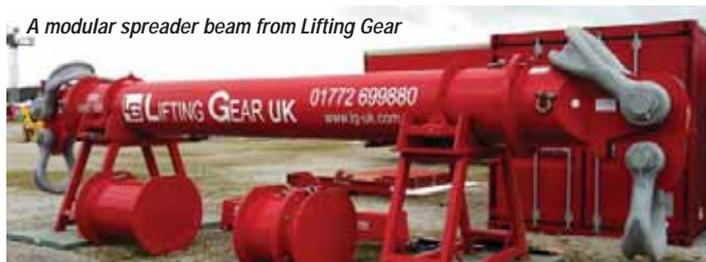
A modular spreader beam from Lifting Gear
