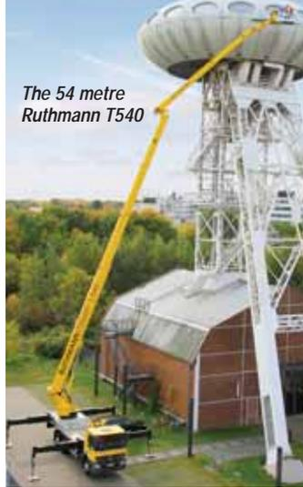
mounted on a 26 tonne chassis - the second model in the company's recently completed Height Performance range.
