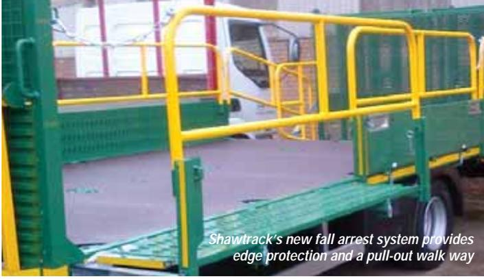
Shawtrack's new fall arrest system provides edge protection and a pull-out walk way
