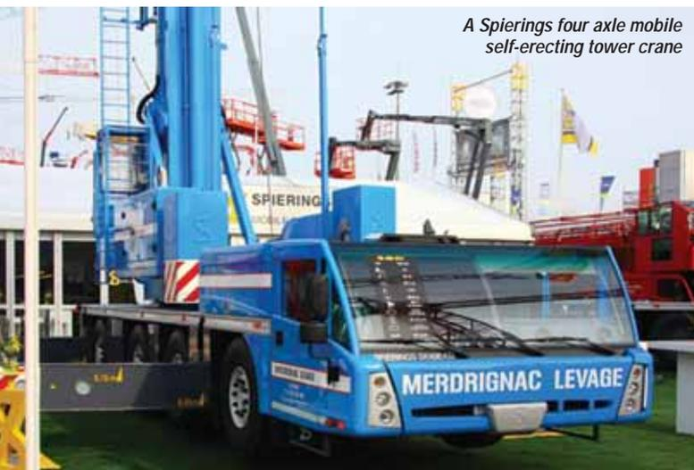
A Spierings four axle mobile self-erecting tower crane
